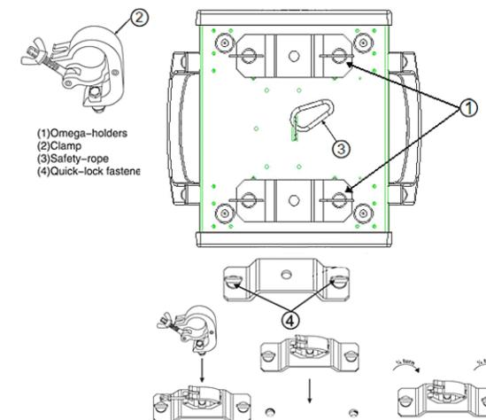
Regardless of the rigging option you choose for your SPOT LED, always be sure to secure your fixture with a safety cable. The fixture provides a built-in rigging point for a safety cable on the hanging bracket as illustrated above. Be sure to only use the designated rigging point for the safety cable and never secure a safety cable to a carrying handle.
