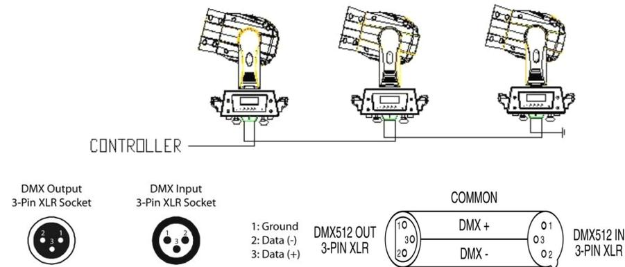
For installations where the DMX cable has to run a long distance or is in an electrically noisy environment, such as in a discotheque, it is recommended to use a DMX terminator. This helps in preventing corruption of the digital control signal by electrical noise. The DMX terminator is simply an XLR plug with a 120 Ω resistor connected between pins 2 and 3, which is then plugged into the output XLR socket of the last fixture in the chain. Please see illustrations below.
